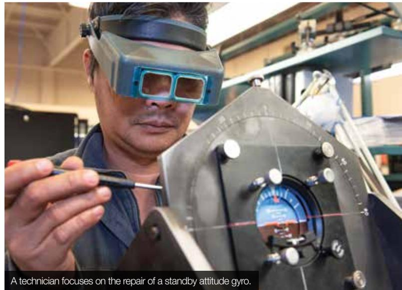
A technician focuses on the repair of a standby attitude gyro.
