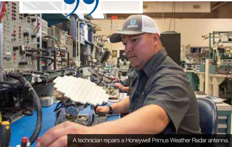
A technician repairs a Honeywell Primus Weather Radar antenna.
