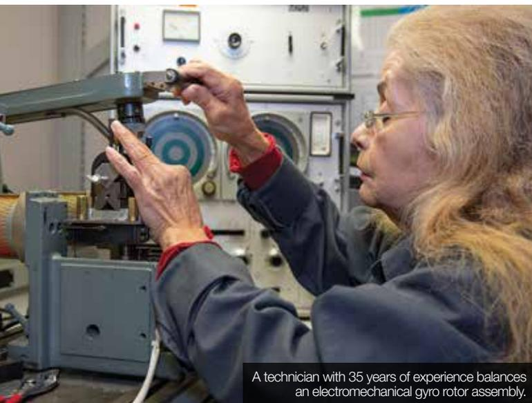
A technician with 35 years of experience balances an electromechanical gyro rotor assembly.
