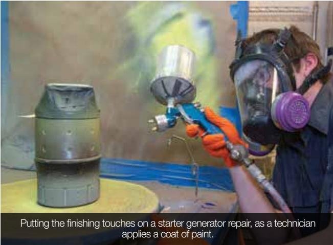
Putting the finishing touches on a starter generator repair, as a technician applies a coat of paint.
